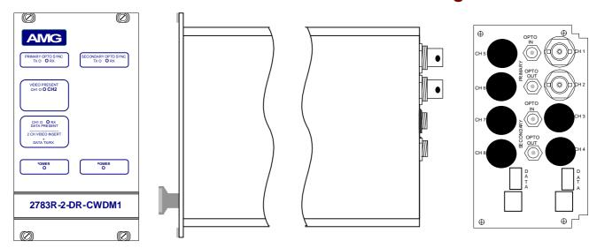
**AMG2783R-2-DR-CWDMn** is a dual channel video insert unit designed to transmit a video signal on to a dual fibre dual redundant optical ring, operating at CWDM wavelength 'n'. It also provides a RS485/RS422 or RS232 bi-directional data channel. The **AMG2783R-2-DR-CWDMn** is designed to plug into an **AMG2000** or an **AMG2005** subrack which in turn fits into a 19" rack system.
