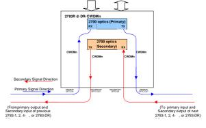
the signal route is not OK. The previous unit will then send out the data signal on its secondary output. This signal will be repeated around the ring to get back to this **AMG2783R-2-DR-CWDMn.** on the secondary route. As the primary input is not present on this unit, the data signal will now be taken from the secondary optical input. Thus maintaining integrity of the video and data transmission.
